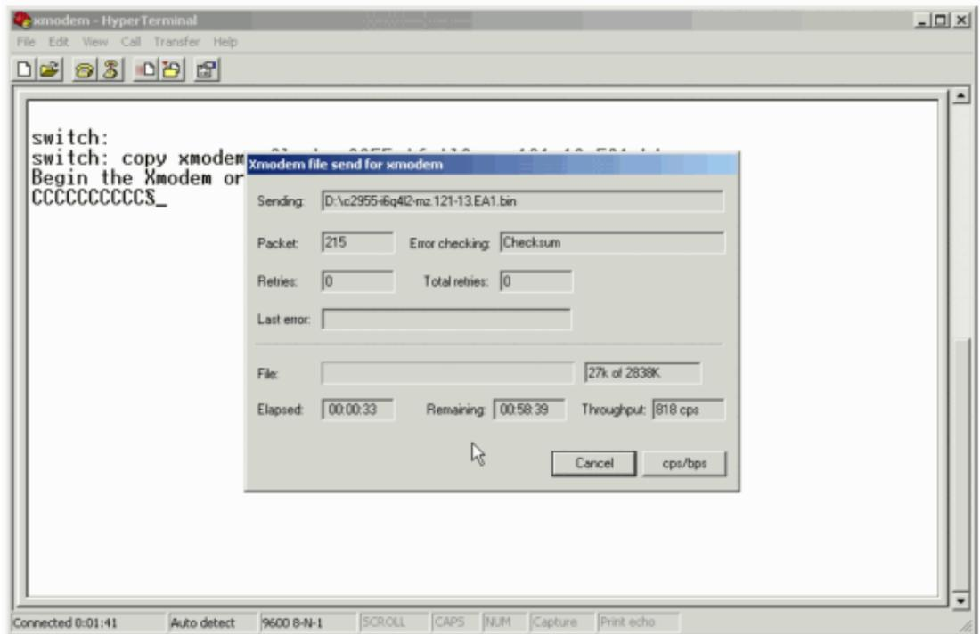
The Xmodem file transfer begins. This transfer can take up to 2 hours, which depends on the size of the image.
